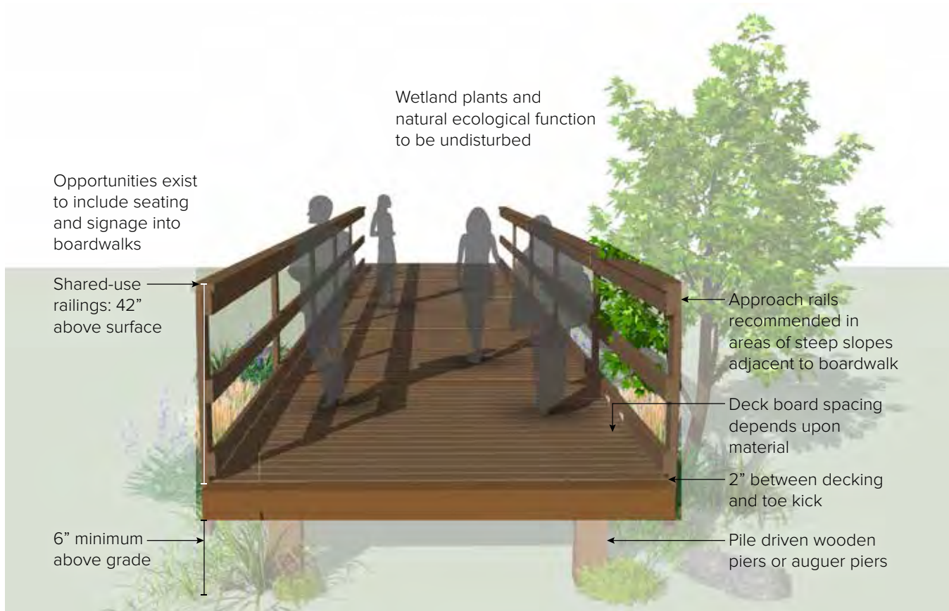
FIGURE 4G Typical bridge/boardwalk cross-section.
